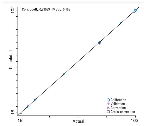
Figure 5: Calibration result for a 60° ARK ATR biodiesel blend
