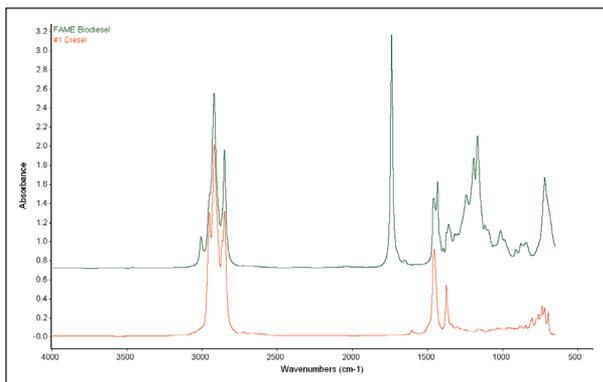
Figure 2: Spectrum of a #1 Diesel and FAME
