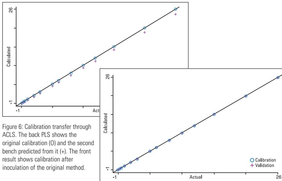
Figure 6: Calibration transfer through ACLS. The back PLS shows the original calibration (O) and the second bench predicted from it (+). The front result shows calibration after inoculation of the original method.
