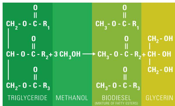
Figure 1: The chemistry of transesterification
